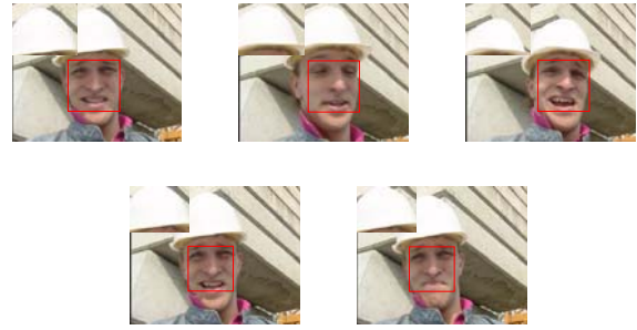
Figure 4. Face detection results. The sub-image at the left-upper corner shows the region right above the face (in this sequence, it is the hard hat region).
