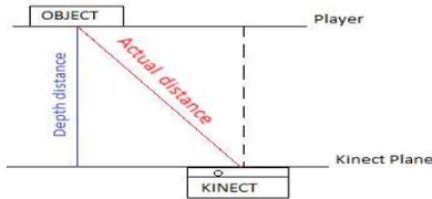
Figure 3. This figure shows that the depth is an estimate of the distance from the object to the camera-laser plane rather than the actual distance from the object to the sensor.
