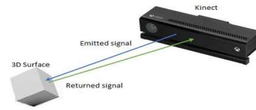
Figure 4. Time of Flight (TOF) of Kinect sensor
