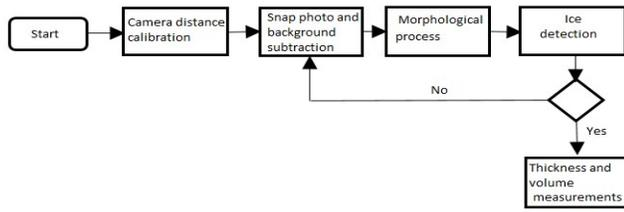
Figure 2: Vision detection approaches using depth camera.
