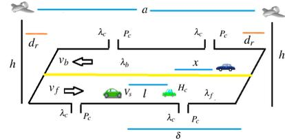
Fig. 1: System model for the considered highway.
