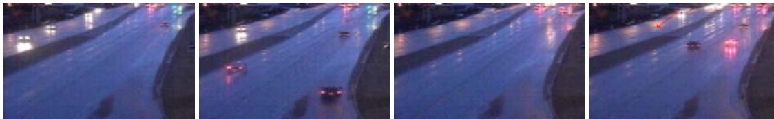
Figure 1: False alarm caused by glare on a wet road
