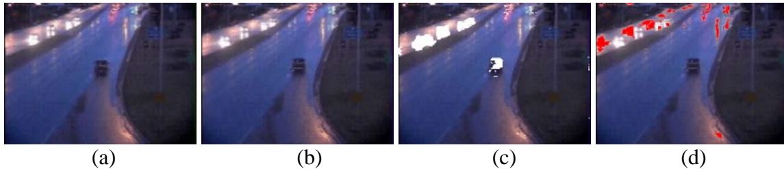
Figure 3: Results (a: previous frame, b: current frame, c: motion detection, d: glare map)
